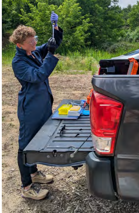
At left: Stephanie Baklarz, research scientist with Wave Lumina, testing PFAS levels in the field with the PFAS field sensor prototype under development. At right: Wave Lumina CEO Vernon Lalone with the PFAS field sensor prototype.
