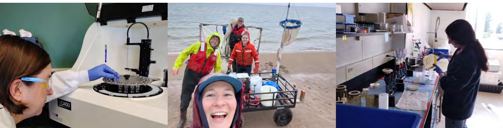
At left , Rima Upchurch (CIGLR) operating a SEAL Analytical AQ400 discrete analyzer to measure nutrient concentrations in water, such as phosphorus, nitrogen, or other chemical parameters. Middle , Maddie Tomczak (CIGLR, front), Cory Brant (USGS, middle, left), Lindsie Egedy (USGS, middle, right), and Greg Faneuff (USGS, back) collect ultraviolet light data from Lake Michigan’s lake whitefish nursery habitats to investigate how sunlight exposure may affect young fish during their critical larval development stage. At right , Brianna Ellis (CIGLR) filters lake water to measure total suspended matter and carbon, hydrogen, and nitrogen content, which help scientists understand water quality and ecosystem health. All photos, courtesy of the Cooperative Institute for Great Lakes Research.
