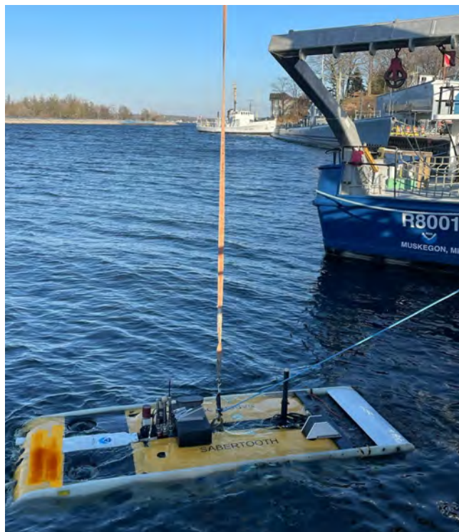
Testing deployments of an autonomous underwater vehicle in Lake Michigan, with the ultimate goal of using it under lake ice during winter to collect ecological and water quality data. Photo credit: Gabrielle Farina, NOAA Great Lakes Environmental Research Laboratory.
