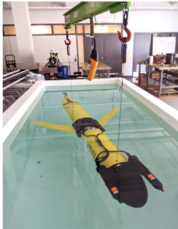
Above, a glider with VR2C acoustic receivers being prepared for deployment in RAEON's test tank. This project tested a mobile platform to track fish movements in the Great Lakes in real time with acoustic telemetry. Photo credit: Cailin Burmaster, AUV Technician.
