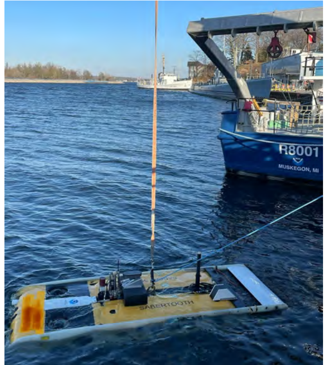
Testing deployments of an autonomous underwater vehicle in Lake Michigan, with the ultimate goal of using it under lake ice during winter to collect ecological and water quality data. Photo credit: Gabriel Farina, NOAA Great Lakes Environmental Research Laboratory.
