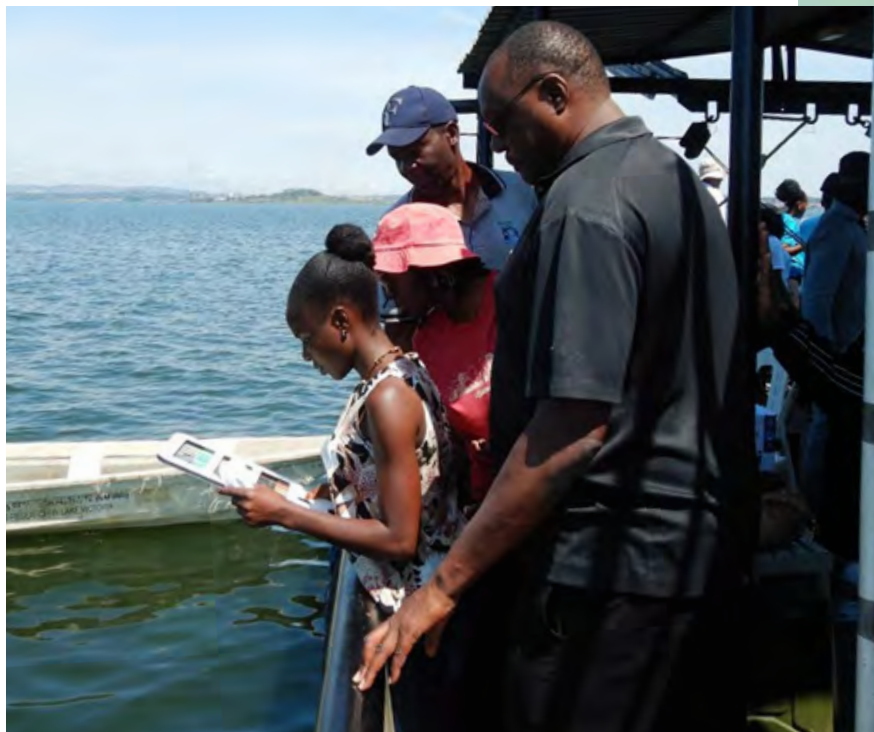
Future water quality experts undergo practical training of determining the color of water using a classical tool, the Forel-Ule scale. Photo by Shungu Garaba.
