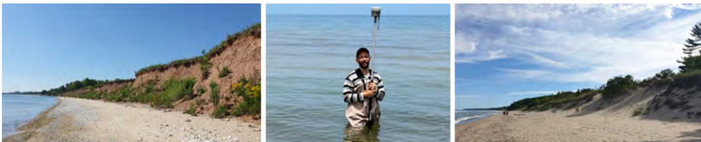
From left, Two Creeks, Wisconsin, author conducting real-time kinematic (RTK) survey at Ogden Dunes, Indiana, and Warren Dunes, Michigan. RTK surveys are used to correct for common errors in satellite navigation systems.
