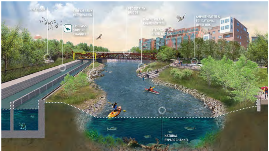
Rendering of FishPass looking upstream with focus on the fish-sorting channels (left) and nature-like bypass channel (right). The bifurcated design enables dual research and recreational access to the Boardman/Ottaway River.
