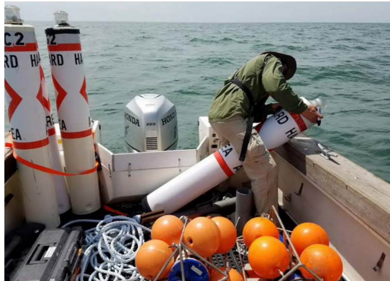
Deploying passive acoustic recording devices in Lake Erie. Photo courtesy of LimnoTech.
