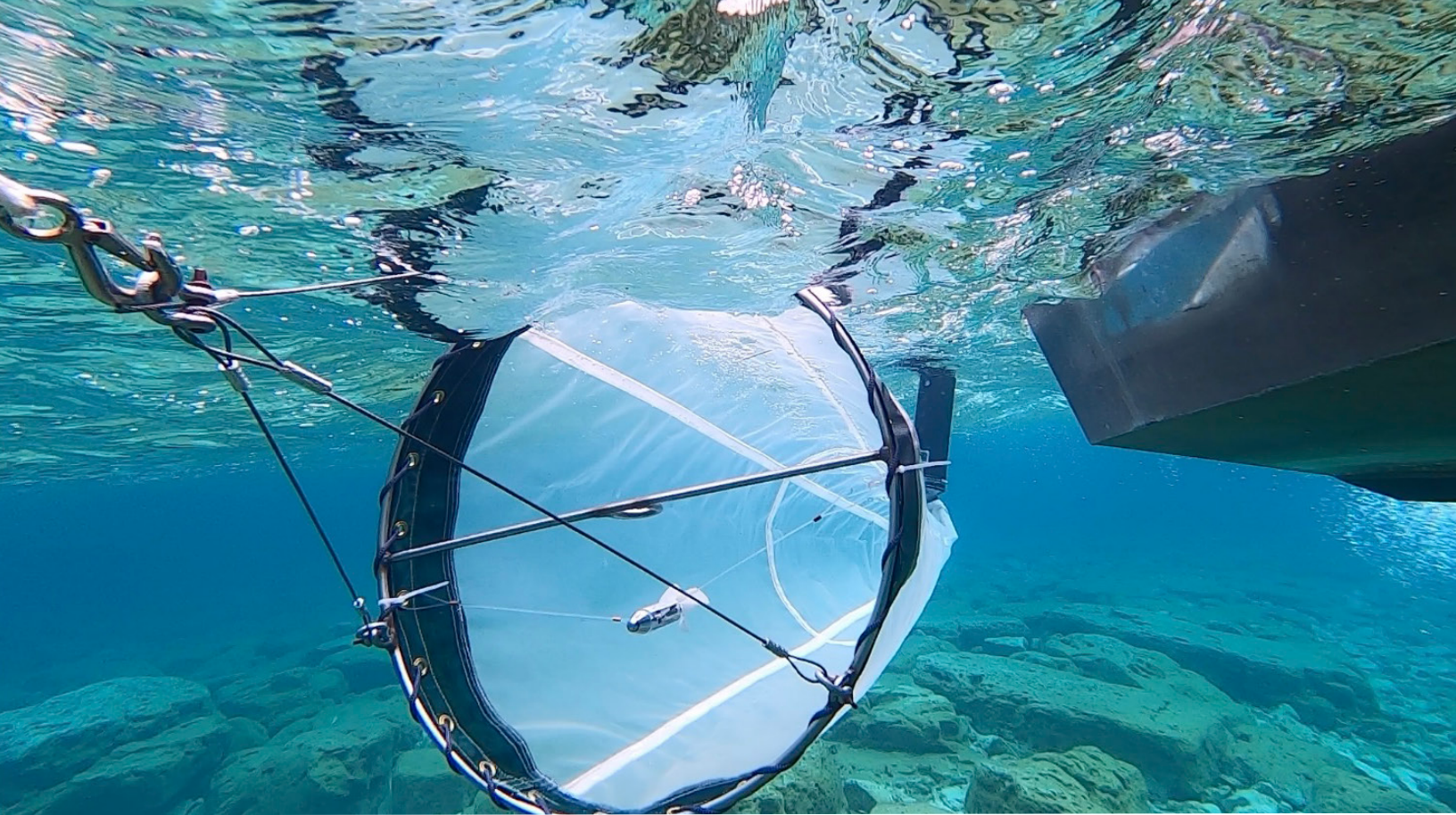
Deployed larval fish sampling net being towed alongside the boat within Lake Huron. All photos courtesy of CWMP.
